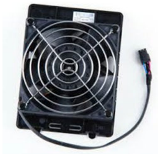
Semipassiver Chassis-Kühler (HP ProLiant ML110 Gen9)
